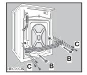
5. Remove the bracket **D** and tighten up the six smaller bolts **C**.
